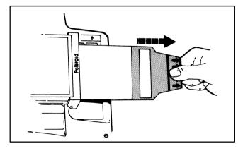
3 Pull the yellow tab, keeping the tab perpendicular to the camera. Position the camera and pull the tab as described in 2 above. A smooth, straight pull will prevent blemishes in the picture.
